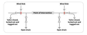
Drain valves must be closed, tagged out, but never locked out.
